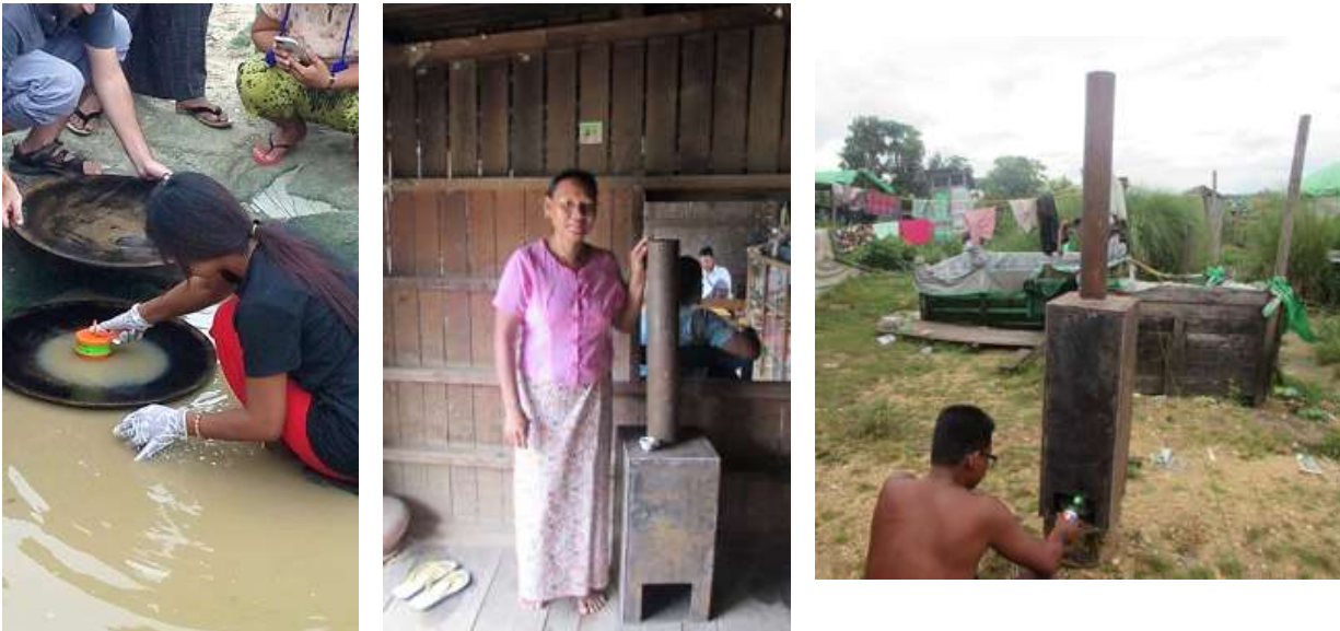
Figure 18. Pact introduced the use of hand magnets to clean mineral concentrates, and co-designed fumehoods with Homalin gold miners.
