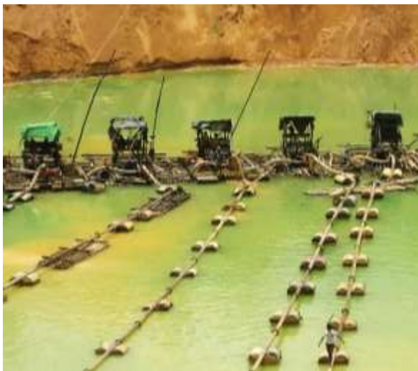
Figure 6. Suction pump dredge mining for gold in Homalin: a miner carefully walks along the 6-inch steel pipe
