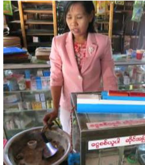
Figure 13 Female mine owner and gold trader refines gold with blow torch to 95 - 98% purity
