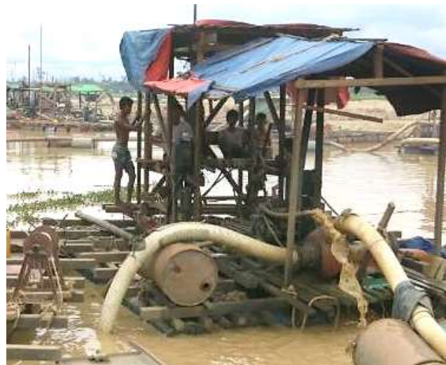
Figure 7. ASM safe and efficient technological advancement. Miner on the left invested in mechanical spud driver to increase production, improve safety and increase profitability
